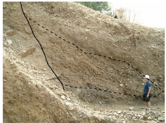
Figure 3. Photograph of a colluvial wedge at the Mapleton Megatrench. The solid and the dashed lines delineate the fault plane and the colluvial wedge, respectively.
