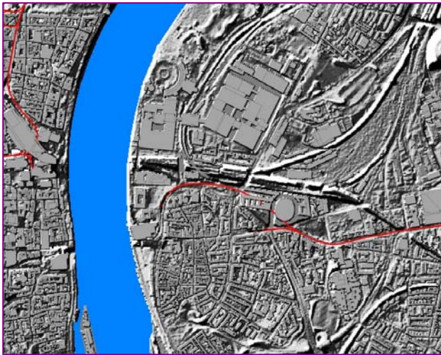
Fig. 6: High resolution DEM underlying the hydraulic model HWSZ (left) and inundation scenario of the model DFNK for water level of 11.29 m at gauge Cologne (bottom).
