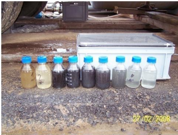
Fig. 2: Visual observation of first the 5 \text{m}^3 water produced by the \text{N}_2 -lift.
