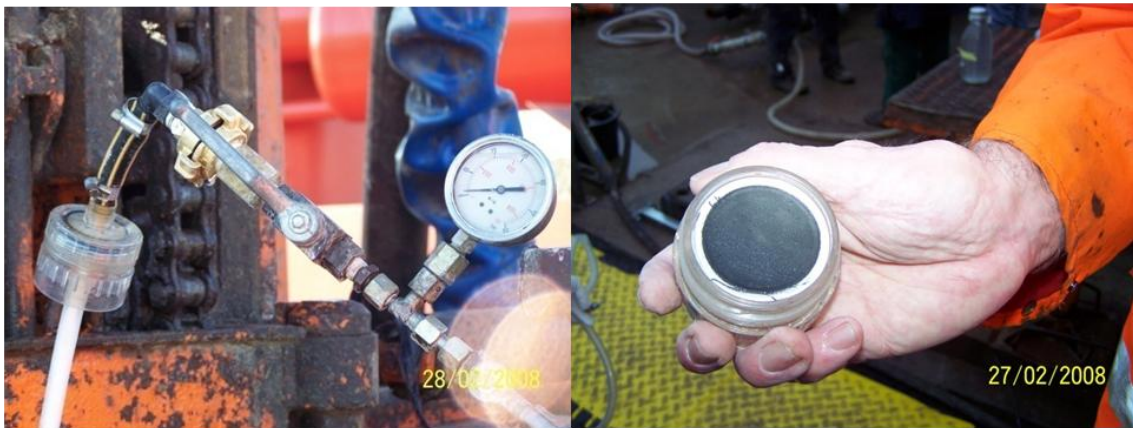
Fig. 3: Membrane filtration of produced water from the \text{N}_2 -lift.
