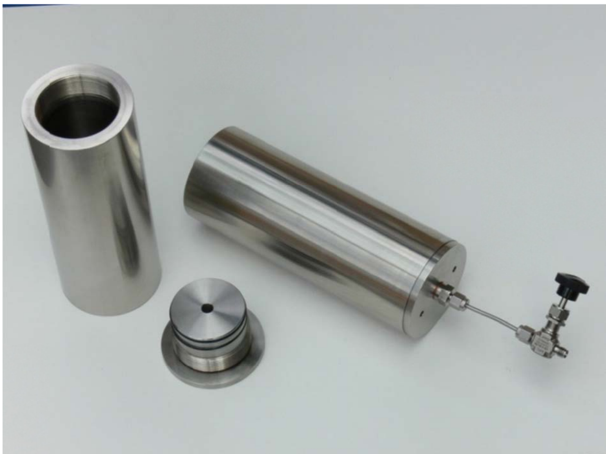
Fig. 2 Corrosion-resistant, high-pressure vessels with a gas valve for cores, with an inner diameter of 60 mm and a length of 140 mm, designed for pressures up to 10 MPa.
