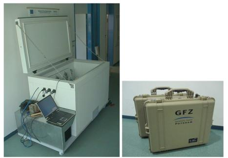
**Figure 2:** *Edgeways and top view of the first set-up of the DAFGAS analytical unit* Main components inside the water vapour tight and air conditioned box are the mass spectrometer with a PC, a pump and a data logger. For details see the technical annex, section A 1.1.
