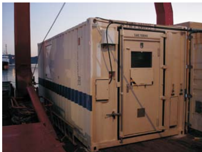
Figure 3. The GFZ BUGLab container is a mobile field laboratory for geomicrobiological and biogeochemical research. The container can be deployed in a wide range of both marine and terrestrial settings, from polar to tropical environments.
