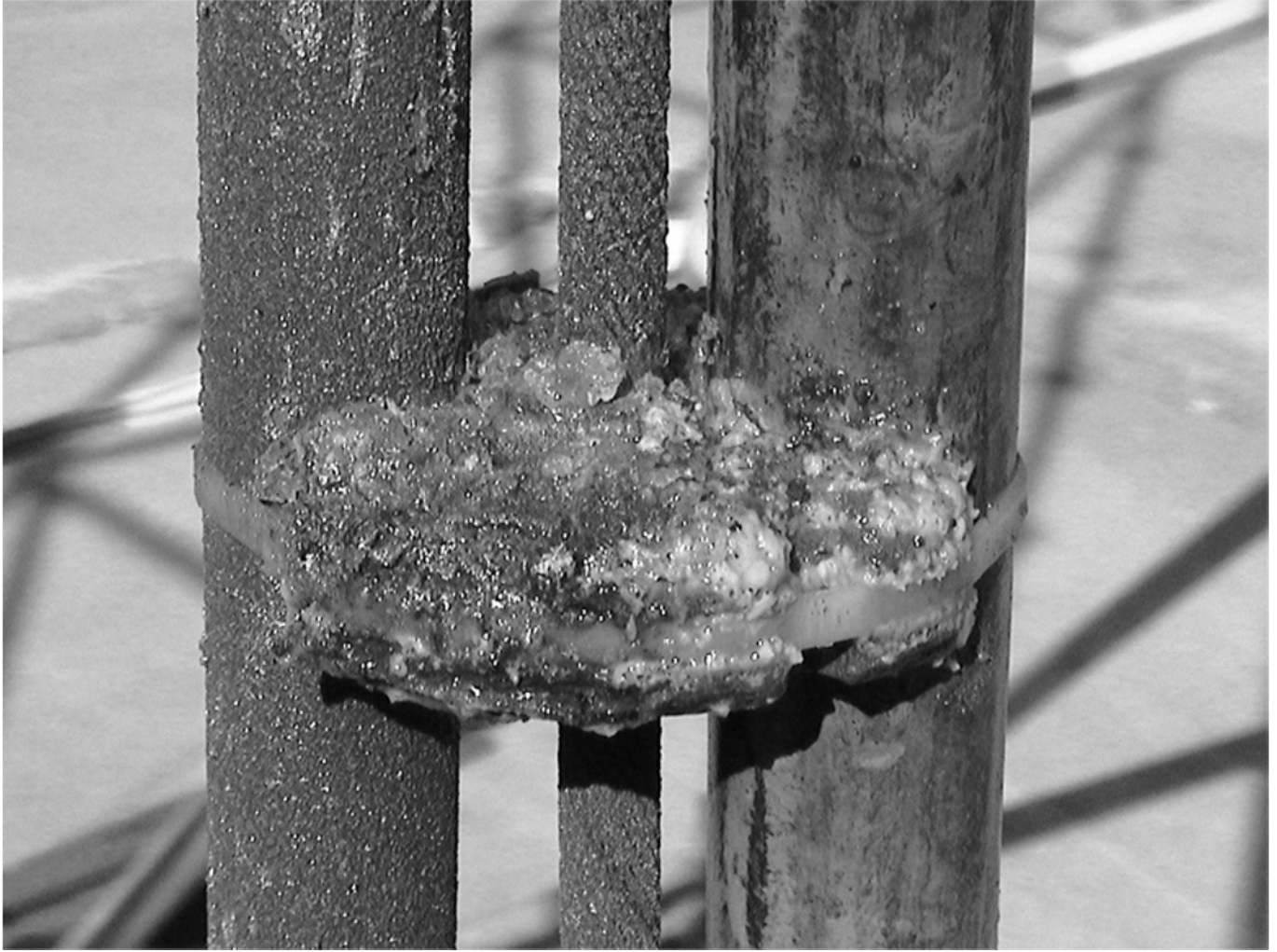
Figure 5: Lead containing scales near the pump in the Groß Schönebeck well (Germany).
