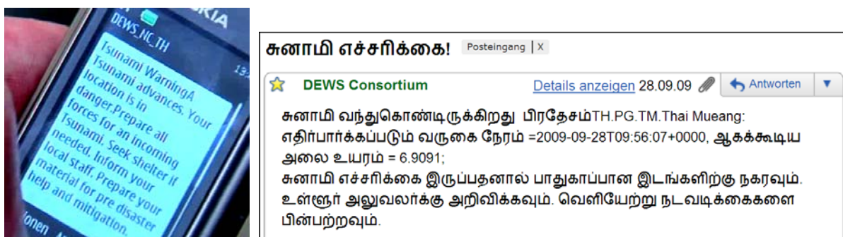
Figure 8. Examples of generated tsunami warnings during live DEWS demonstrations. a: SMS in the English Language informing local rescue services with basic instructions. b: email in the Tamil language including geocode, estimated time of arrival and estimated maximum wave height for the affected territory.
