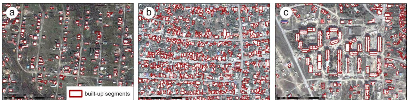
Figure 7. (a) Detached single buildings detected and outlined by built-up mask; (b) Appearance of complex urban settings with attached buildings in built-up mask; (c) Large buildings in built-up mask.
