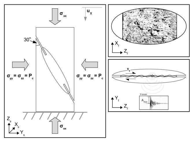
**Figure 1.** (left) Schematic diagram of loading conditions and stresses. Arrows at bottom left specify the sample-specific coordinate system. (right) Sliding of fault with naturally developed roughness in fault specific coordinate system which is also used for the later AE representation.
