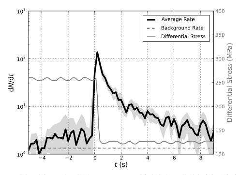
**Figure 4.** Differential stress (gray line), AE rate average (black line), standard deviation (shaded gray region), and background rate (dashed gray line) for all slip events of WGR01, WGRN04 and WGRN05 within a 15 s time window of slip onsets, stacked to t = 0. The origin times of slip events were determined from the stress drop onsets and compared to AE data. The highest AE rates occurred within less than 100  $\mu$ s of the stress drops.
