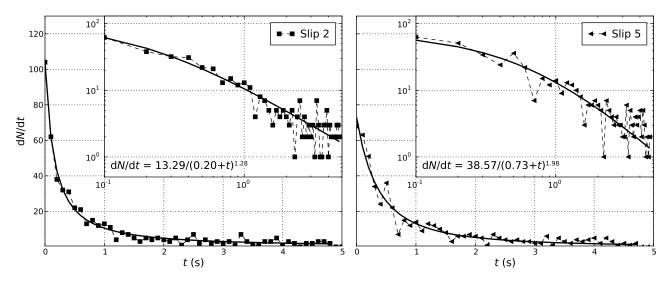
Figure 7. AE aftershock rates for slip events 2 and 5 plotted in linear and logarithmic scale.
