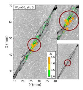
**Figure 14.** CT scan and AE hypocenters colored according to magnitude for foreshocks to slip event 5 of WGRN05. Most of the AE activity is concentrated within the asperity region indicated by a red circle.
