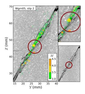
**Figure 13.** CT scan of central part of sample obtained after the experiments and AE hypocenters (colored dots) for the stick periods before slip event 2 of WGRN05. The colors of hypocenter locations correspond to their magnitudes. The red circle highlights the likely site of a large asperity which was centered at [27,45].
