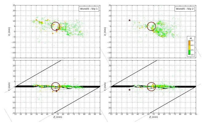
**Figure 9.** Examples of AE foreshock activity based on slip events 1 and 2 of WGRN05. The red circle highlights an area of a relatively sharp contrast between low and high AE activity. Many large amplitude events were produced in the periphery of this area before each of the slip events.
