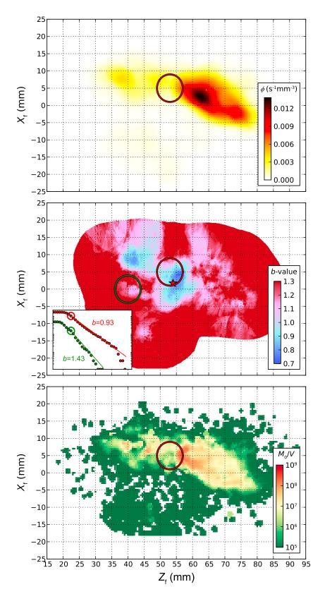
**Figure 10.** Examples of AE event density  $(\phi)$ , b value and moment release maps computed for AEs occurring before slip event 1 of experiment WGRN05. Slip event one (red star) nucleated close to or from within an area of high  $\phi$ ,  $M_0$  and low b value. The finds for high and low b value regions are compared (bottom left in Figure 10 (middle)). The asperity region is connected to low b values, high event density and moment release.
