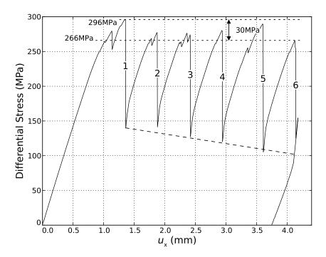
**Figure 2.** Differential stress and axial displacement  $(u_x)$  for experiment WGRN05 with characteristic stick-slip behavior. The slip events with large stress drops are labeled from 1 to 6. All slip events with large stress drops nucleated within a differential-stress window of 30 MPa (dashed lines at top). The residual stress decreased systematically after each successive stick slip as indicated by the downward sloping dashed line.
