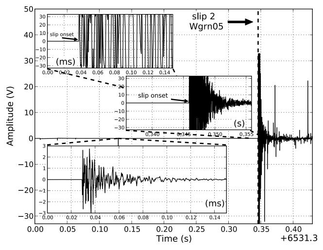
**Figure 3.** AE waveforms within a  $\sim 0.5$  s (main axis), 20 ms (middle) and 0.15 ms (inset at top) time window of slip event 2 of experiment WGRN05 as well as a waveform of a "typical" AE event (inset at bottom). The waveforms connected to slip onsets were clearly distinguishable from commonly observed AEs by their amplitude and duration. Note that time scales are in ms for the top and bottom insets.
