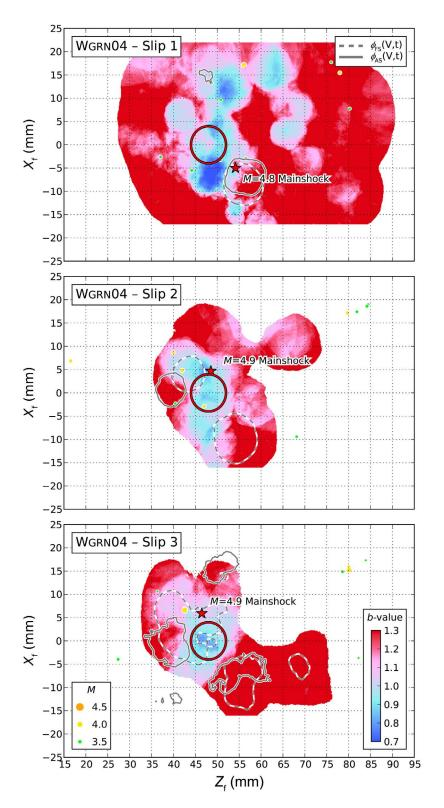
**Figure 12.** b value, foreshock and aftershock densities, main and largest aftershock locations plotted similarly to Figure 11 but now for three different slip events of experiment WGRN04. A combination of b value maps, AE event densities and foreshock locations enables the identification of an asperity region (red circle) which is also the nucleation spot of macroscopic slip events.
