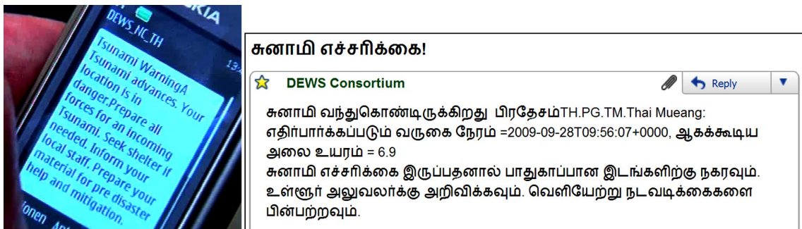
Fig. (15). Examples of generated tsunami warnings during live DEWS demonstrations. Left: A text message in English informing local rescue services using basic instructions. Right: email in Tamil including geocode, estimated time of arrival and estimated maximum wave height for the affected territory.
