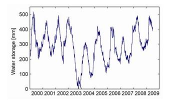
Figure 2: Water storages estimated from superconducting gravimeter. Water storage is expressed using the minimum observed water storage of the study period as the baseline.
