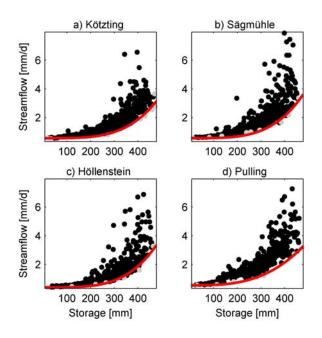
Figure 4: Relation between water storage and streamflow for the four different stream gages (a) Kötzting drainage area, (b) Sägmühle drainage area, (c) Höllenstein drainage area, and (e) Pulling drainage area for the whole study period from January 2000 to October 2009. Red lines are the lower envelop curve and black dots are the bin averages.
