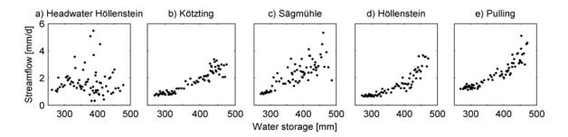
Figure 3: Relation between water storage and streamflow for the five different stream gages: (a) headwater Höllenstein drainage area, (b) Kötzting drainage area, (c) Sägmühle drainage area, (d) Höllenstein drainage area, and (e) Pulling drainage area for the period December 2007 to October 2009. Black dots are the bin averages.
