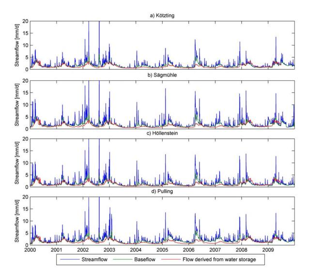
Figure 5: Measured streamflow and estimated baseflow measured at the four different stream gages: (a) Kötzting drainage area, (b) Sägmühle drainage area, (c) Höllenstein drainage area, and (d) Pulling drainage area in combination with the flow derived from SG measurements, using the lower envelop curve of Figure 4 for the storage-baseflow-relationship.
