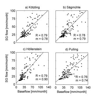
Figure 6: Monthly baseflow in comparison to flow derived from SG measurements (SG flow) for four different stream gages: (a) Kötzting drainage area, (b) Sägmühle drainage area, (c) Höllenstein drainage area, and (d) Pulling drainage area in combination with the regression line (black line), the Pearson correlation (R) and the slope of the regression line (m). All correlation coefficients are below the significance level of p=0.01.
