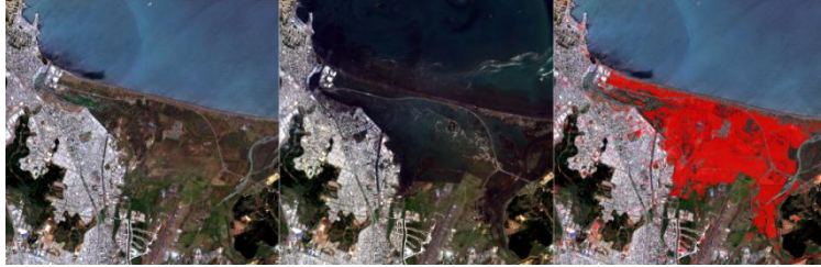
Figure 1. Damages by tsunami: City of Concepcion, Chile imaged on 10/01/2010 (left images) and 27/02/2010 (centre/right images) by the RapidEye satellite constellation. The centre image was taken eight hours after an earthquake of magnitude 8.8 had occurred and the resulting tsunami had affected the shoreline. The right map shows the areas with tsunami-related changes (red layer) on the post-tsunami image. Images courtesy of RapidEye AG, Copyright 2011, all rights reserved.
