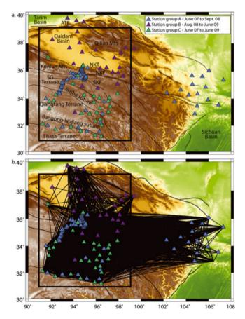
**Figure 1.** (a) Map showing stations for the INDEPTH IV arrays, colored by deployment dates. Stations recording fewer than 10 days of data are omitted. Rectangle encloses the study area shown in Figures 2 and 3. (b) Two-station path coverage actually used in our ambient-noise tomography. Not all stations successfully recorded data during the full deployment of the array. ATF: Altyn Tagh fault; NKT: North Kunlun thrust system; NKF: North Kunlun fault; SKF: South Kunlun fault; SG: Songpan Ganzi.
