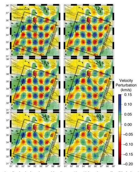
Figure 2. Results of a checkerboard test with columnar  $1^{\circ} \times 1^{\circ}$  lateral anomalies. Black dots indicate stations.
