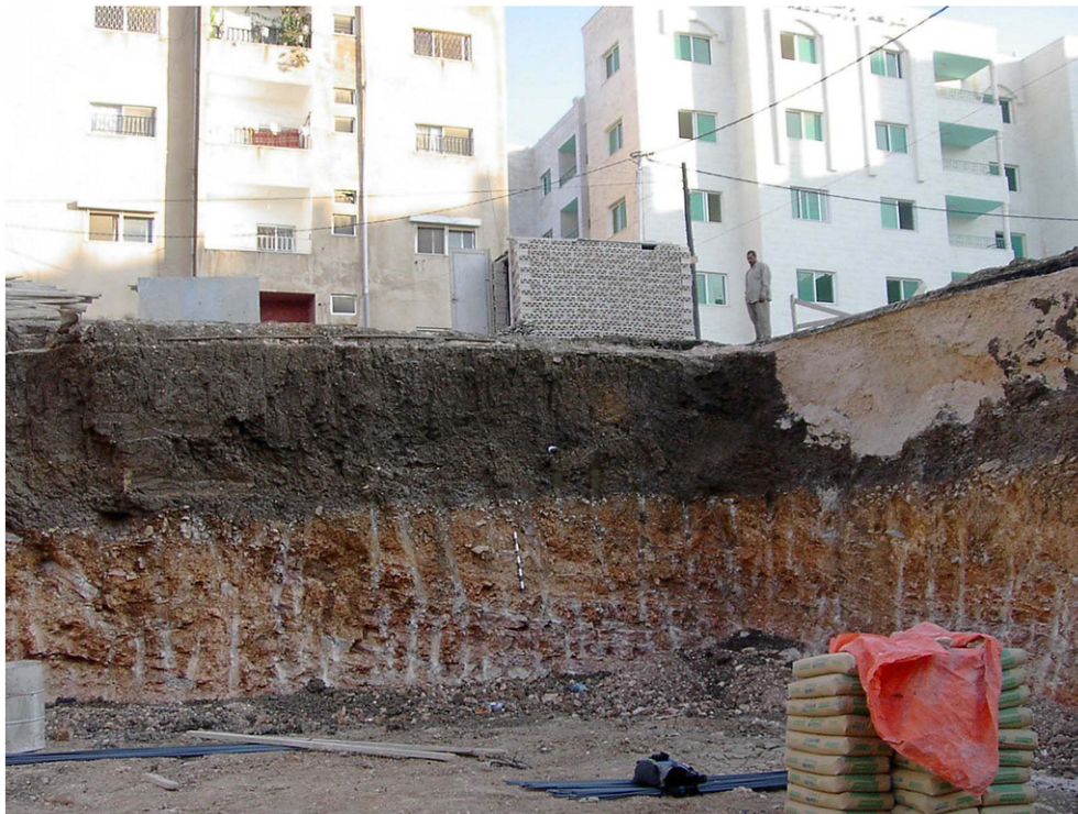
Fig. 6. The Red Mediterranean Soil on silicified limestone revealed by a construction pit in the city of Irbid. Each mark on the metre represents 10 cm. The picture was first published in Lucke (2008, 45) and is reprinted with permission of Akademikerverlag.
