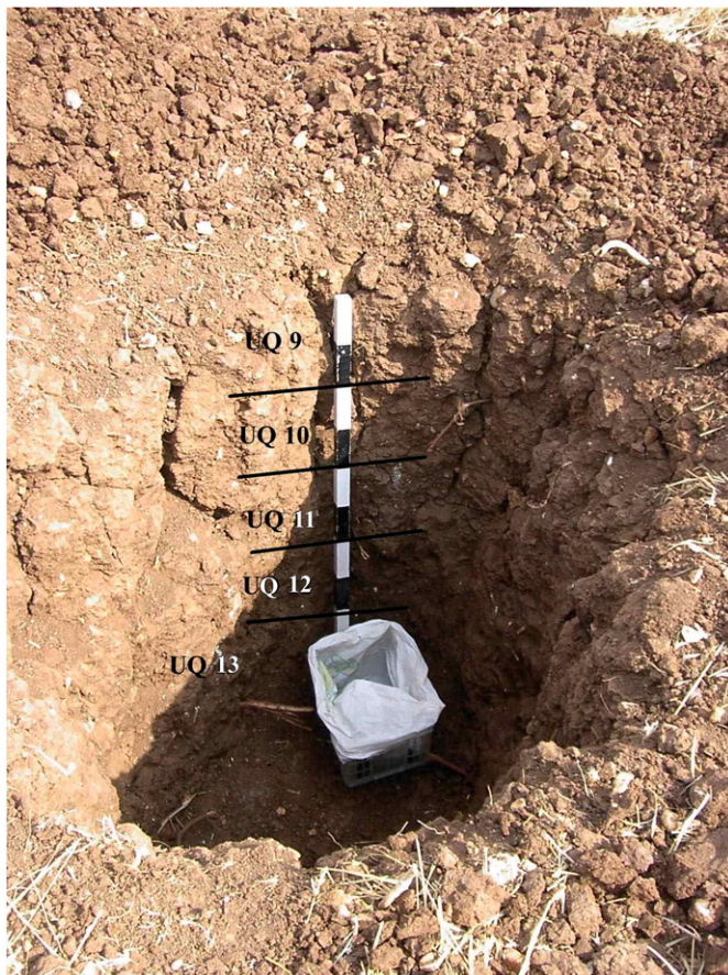
Fig. 3. Sampling the Red Mediterranean Soil on basalt near the village Umm Queis. Each mark on the metre represents 10 cm.
