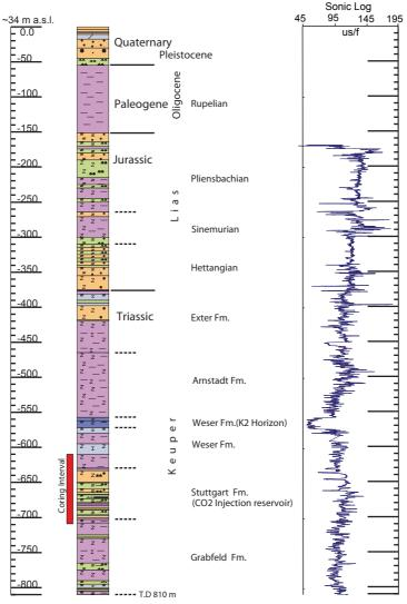
The profile is based on cutting analysis, core description, and log interpretation. Geological interpretation still in process.
