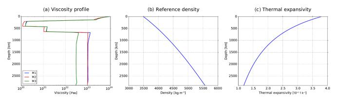
Figure 2. Radial profiles of (a) viscosity, (b) density and (c) thermal expansivity in our models.
