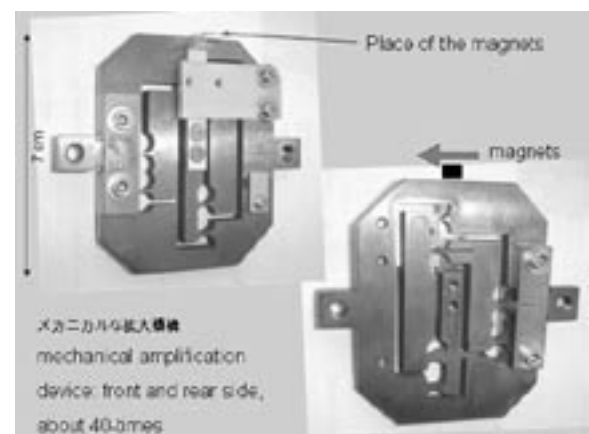
Figure 2: Mechanical amplification device from both sides: The plate is strained between left and right, and the movement of the magnets is monitored.
