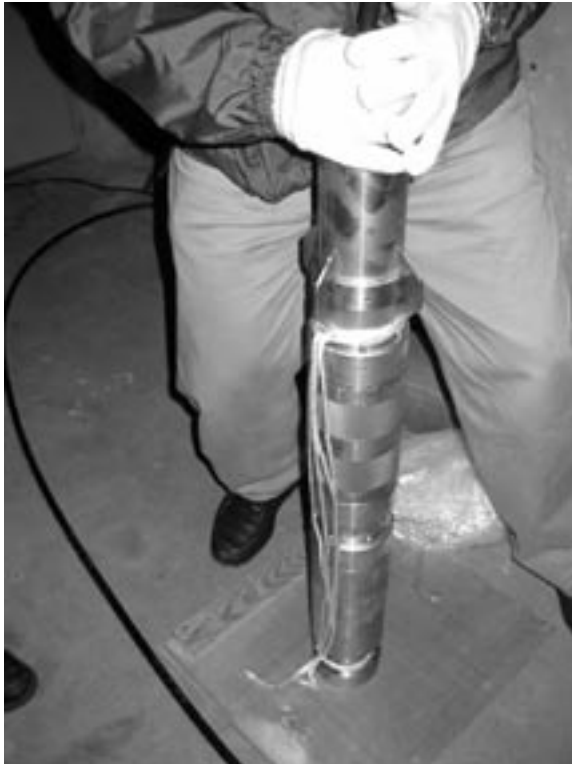
Figure 1: The strainmeter prior to installation.
