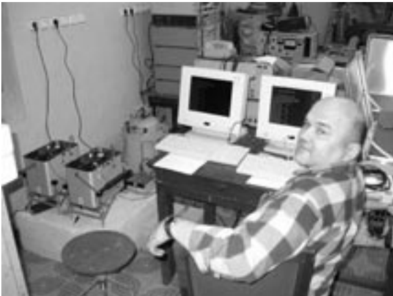
Figure 3: Fig. 3. Both Burris gravimeters (left) and the panel PCs; in front Dr. Kopaev.
