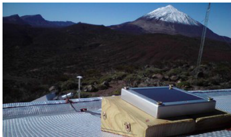
Figure 3: IYA Lightmeter installation at the Teide Observatory at Izaña, Tenerife (Image by Hans Deeg).
