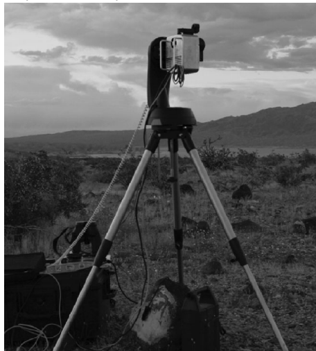
Figure 7: The camera system used by the US National Park Service for all-sky mosaics.
