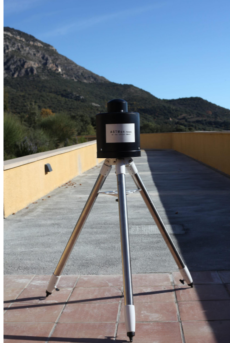
Figure 4: The ASTMON portable (Lite) version without weatherproof system (Image by Ramon Canal-Domingo).
