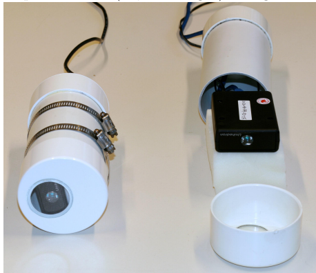
Figure 1: Photograph showing the Sky Quality Meter installed in its protective housing (SQM-LU left), along with an expanded view (SQM-LE right). Image and caption from [52]
