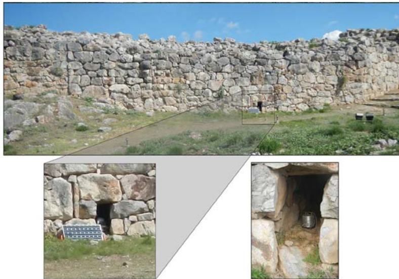
Figure 2: Setting of station HE01 at the Tiryns citadel on hard rock in a drainage channel of the Cyclopean fortification wall. (Photos K.-G. Hinzen)
