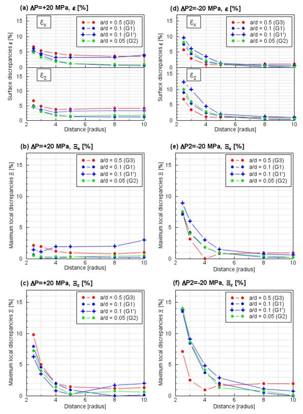
Figure 5. Model B: surface ( $\epsilon$ ) and maximum local ( $\Xi$ ) discrepancies vs source separation, obtained for models combining two juxtaposed spherical sources, one of them being pressurized by  $\Delta P_1 = +20$  MPa and the other one being either pressurized by  $\Delta P_2 = +20$  MPa (left-hand column: a–c) or pressurized by  $\Delta P_2 = -20$  MPa (right-hand column: d–f). Corresponding discrepancies values are listed in Table A-3.
