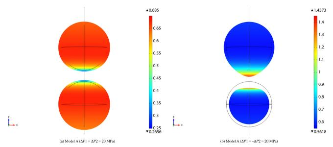
Figure 7. Models A (Group G1'a): Cross-section of the source total deformation (m) of a spherical source pressurized by  $\Delta P1 = 20$  MPa superposed to another spherical source pressurized by either  $\Delta P2 = 20$  MPa (left-hand panel) or  $\Delta P2 = -20$  MPa) (right-hand panel), in an homogeneous medium. The source deformation is magnified by a factor of 100.
