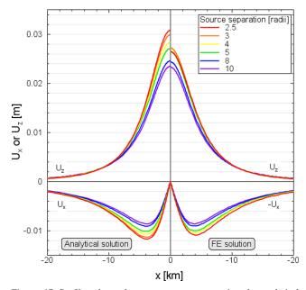
**Figure 17.** Profiles above the source centre comparing the analytical (left-hand panel) and FE (right-hand panel) vertical and horizontal surface displacements for models with two superposed spherical sources (Model A-G1') for source separations between 2.5 and 10 radii. For easier comparison, we mirrored the horizontal displacements of the FE solution.
