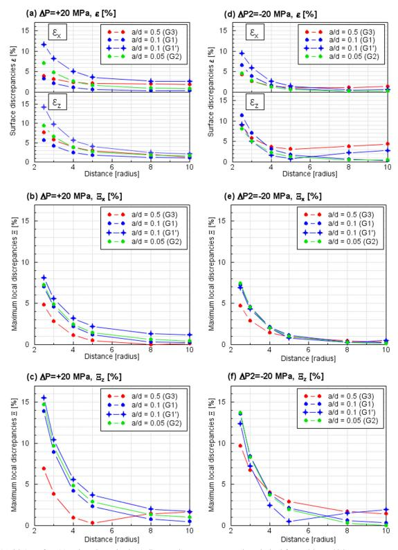
Figure 4. Model A: surface ( $\epsilon$ ) and maximum local ( $\Xi$ ) discrepancies vs source separation, obtained for models combining two superposed spherical sources. The shallower source is pressurized by  $\Delta P_1 = +20$  MPa and the deeper source is either pressurized by  $\Delta P_2 = +20$  MPa (left-hand column: a–c) or underpressurized by  $\Delta P_2 = -20$  MPa (right-hand column: d–f). Corresponding discrepancies values are listed in Table A-2.
