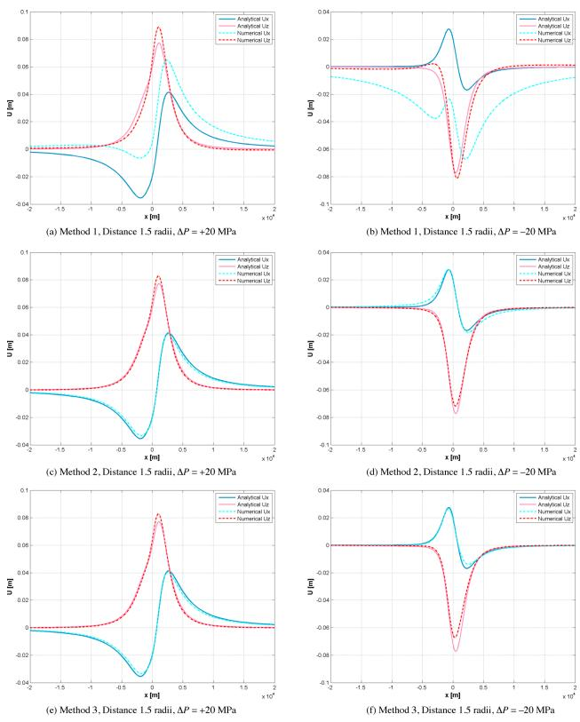
**Figure 9.** Model DIa: surface displacements across the centre of the deformation sources for models of a dyke opening by 1 m, modelled by Methods 1-3, juxtaposed to a spherical source pressurized by either  $\Delta P2 = +20$  MPa (left-hand column: a, c and e) or  $\Delta P2 = -20$  MPa (right-hand column: b, d and f). The sources are separated by a distance of 1.5 radii. The profiles for further source separation are presented in Figs A-4–A-6.
