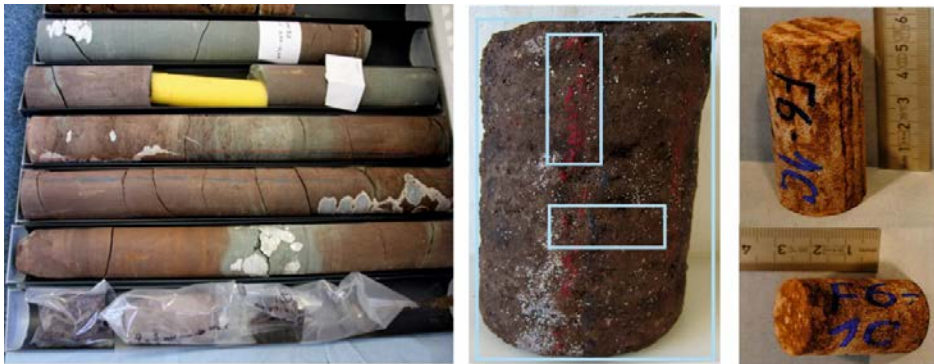
Figure 1: Recovered core material of well Ktzi 203 and prepared plugs for Nitrogen permeability
