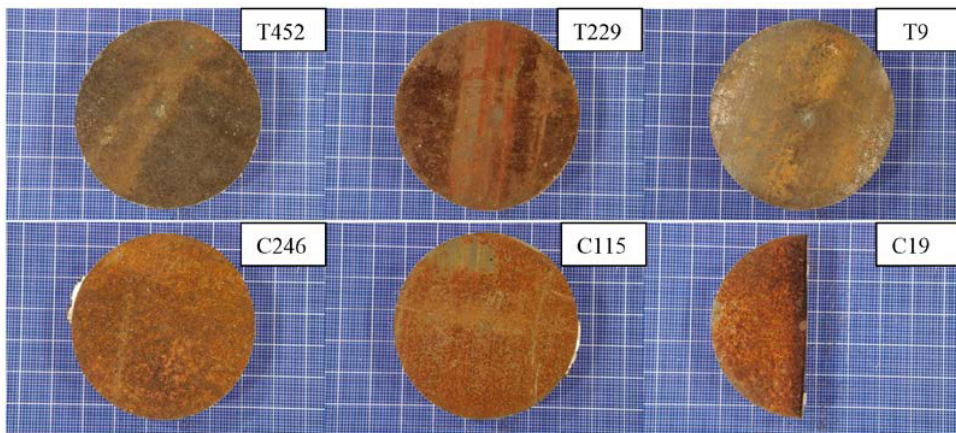
Fig. 13. Images of external surfaces of casing (C) and production string (T) samples retrieved at different depths.
