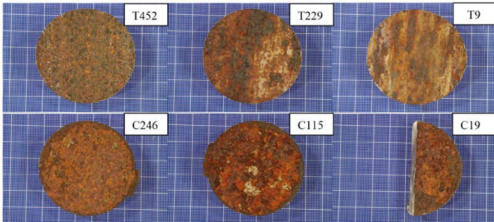
Fig. 12. Images of internal surfaces of casing (C) and production string (T) samples retrieved at different depths.
