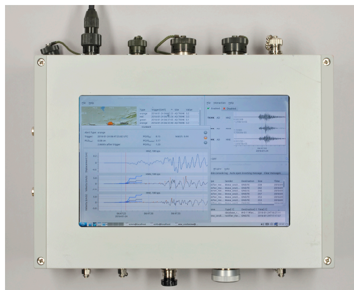
Figure 1. A MPwise unit. This version includes a touchscreen embedded in the housing. While this arrangement is not standard, an external touchscreen can be connected to all units. In this image, the touchscreen display shows the operation of the onsite EEW software described in [5–7]. The dimensions of the latest version are: length 20.5 cm, width 16 cm, and height 8 cm.
