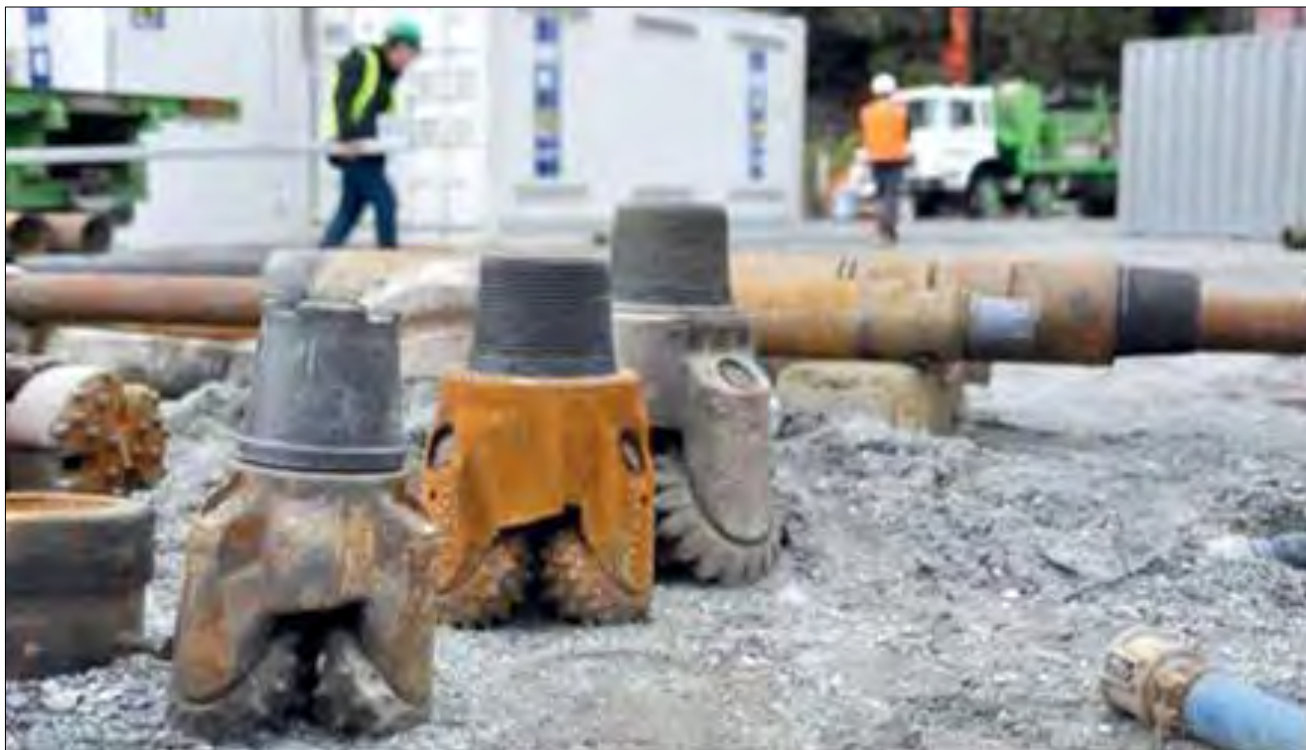
Figure 3: Drill bits at the Alpine Fault drill site, New Zealand
