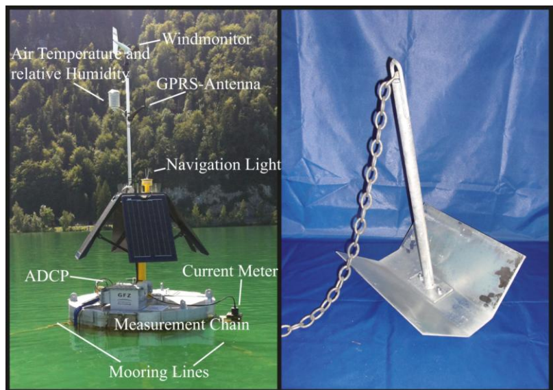
Figure 2. Buoy in operation and plate anchor as used for the mooring.
