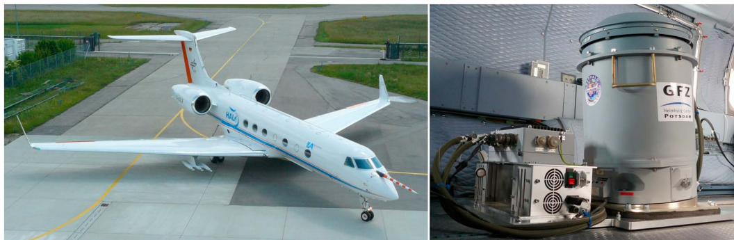
Figure 1. Equipments of airborne gravimetry of the GEOHALO mission: (left) the High Altitude and Long Range (HALO) aircraft and (right) the Airborne/Marine Gravimeter Chekan-AM.
