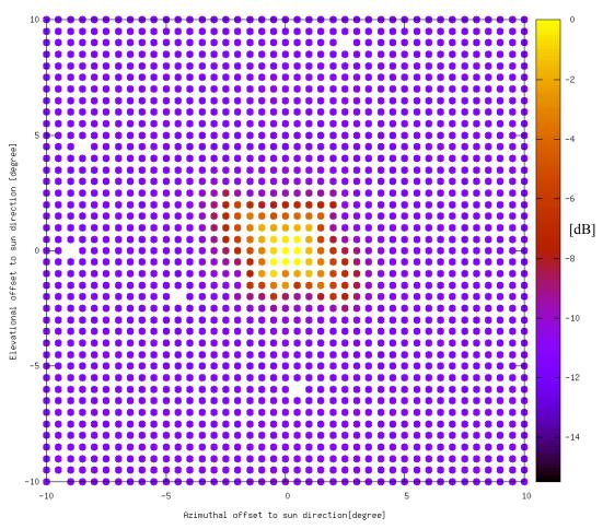
Figure 84: NYA-2 directivity with boresight offset compensation, square scan, 0.5° steps
