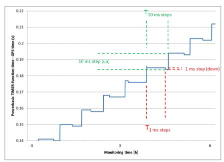
Figure 60: Closer view on PC system time drift
