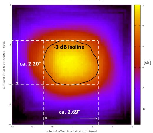
Power of detected sun noise, relative to maximum [dB]
