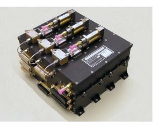
instrument uses a GPS signal tracking Figure 9: IGOR GPS-receiver (© GFZ) mechanism ("open loop tracking") that
