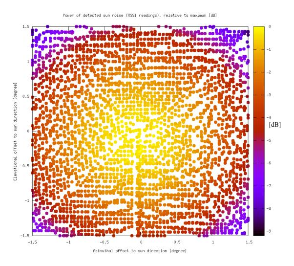
Figure 78: NYA-1 directivity with boresight offset compensation, square scan, 0.05° steps
