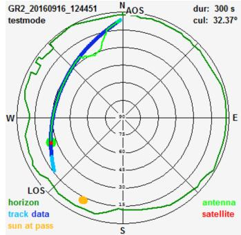
The antenna trace must be expected to be in perfect alignment with the pre-calculated satellite track (blue colours). A temporary wrong antenna positioning in the azimuth interval between 126
