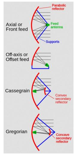
parabolic reflector antennas
