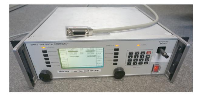
Figure 42: Antenna control unit (ACU) for NYA-1 antenna system
