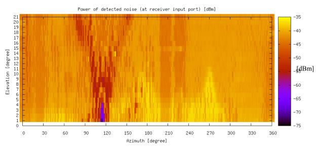
Figure 91: First scan of horizon with NYA-1 antenna (resolution Az = 0.5°, El = 1.0°)
