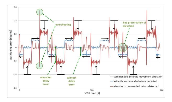
Figure 80: Analysis of positioning errors during square scan (0.5° steps) with NYA-1
