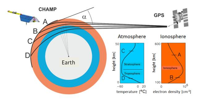
Figure 4: GPS-based sounding of atmosphere and ionosphere (adopted from Wickert 2002)
