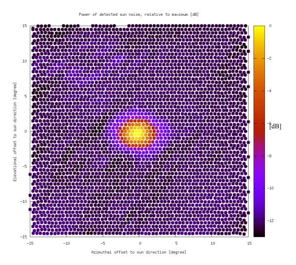
Figure 88: NYA-1 directivity with boresight offset compensation, stripe scan, 0.5° steps
