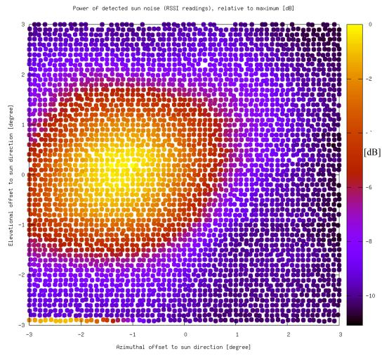
Figure 81: NYA-2 directivity w/o boresight offset compensation, stripe scan, 0.1° steps
