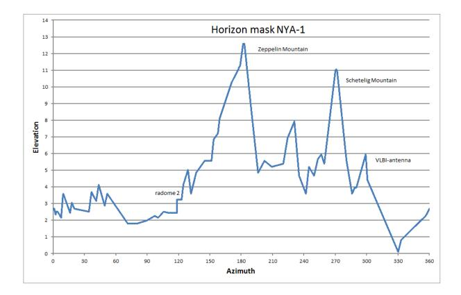
Figure 49: NYA-1 antenna horizon mask
