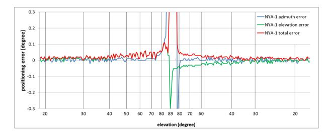
Figure 97: Tracking performance of NYA-1 during pass with 89° culmination
