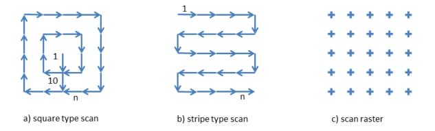
Figure 53: Movement schemes and raster of scan functions
