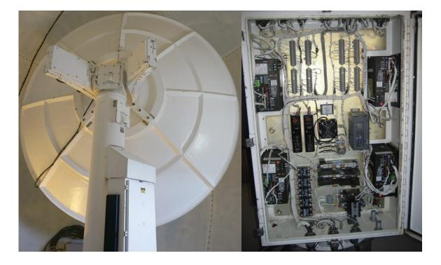
Figure 41: NYA-1 antenna system and drive electronics cabinet
