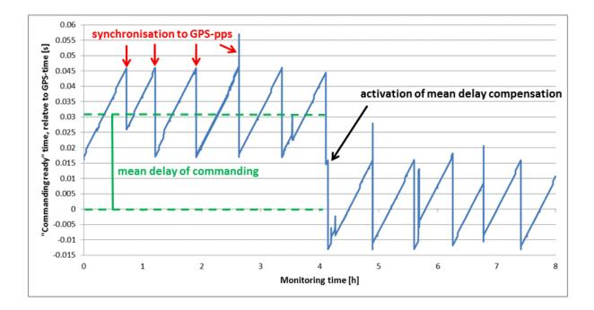
Figure 63: Timing accuracy of antenna commanding
