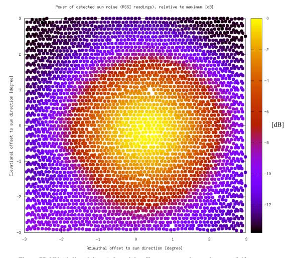
Figure 77: NYA-1 directivity w/o boresight offset compensation, stripe scan, 0.1° steps
