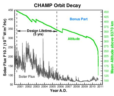
Four orbit rise maneuvers were with performed CHAMP between 2002 and 2009 to compensate the unwanted fast orbit decay from an unexpected high solar activity as well to extend the as planned mission life time (Figure 12). orbit thrusters The on CHAMP were operated during
