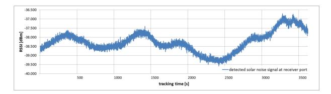
Figure 72: Variation of solar radio noise signal (S-band) from exemplary measurement
