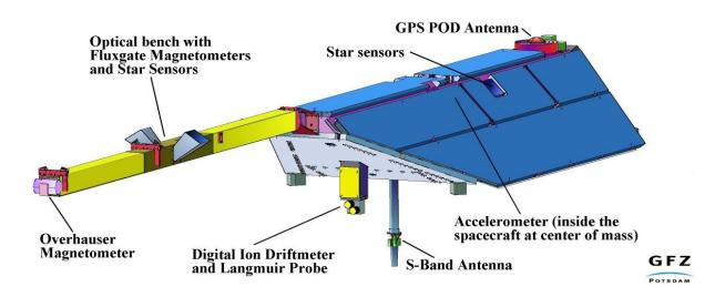
Figure 3: Instruments on satellite CHAMP (© GFZ)
