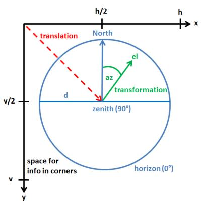
Figure 55: Construction scheme of NYA-Sattrack skyplot display
