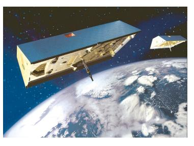
the GRACE satellites is very similar to the design of CHAMP and includes special GPSequipment (POD and GPS-RO), star-sensors (attitude determination) and accelerometers for the measurement of non-gravitational forces, but no magnetometers and instrument boom and no instruments for electric field measurements. Irregularities in the Earth's gravity field affect the orbits of the satellites, one after the other, and thus also the distance between the satellites.
