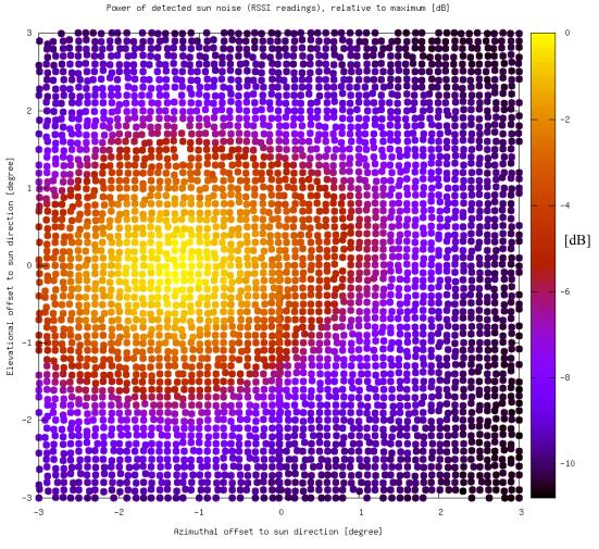
Figure 82: NYA-2 directivity w/o boresight offset compensation, square scan, 0.1° steps
