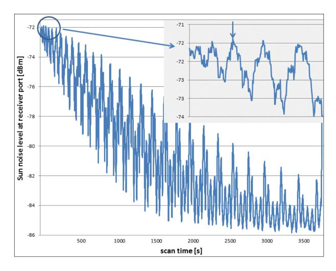
Figure 70: Sun noise during first experiment with NYA-1 (square-type scan)
