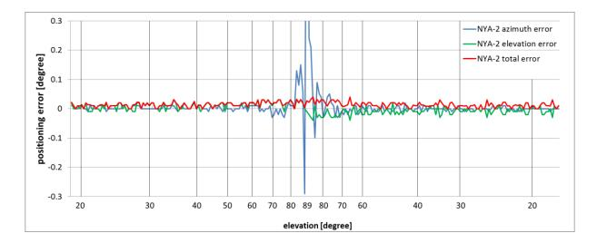
Figure 98: Tracking performance of NYA-2 during pass with 89° culmination
