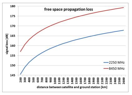
Usually such calculations Figure 29: Free space propagation loss in S-band and X-band
