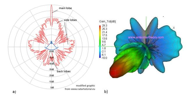
Figure 27: Examples of parabolic antenna radiation pattern
