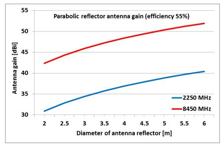
with the antenna Figure 30: Antenna gain in S-band and X-band w.r.t. antenna size reflector diameter.
