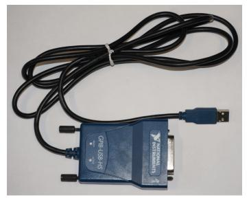
standard USB computer interfaces to Figure 54: USB to GPIB (IEEE-488) adapter from National IEEE-488 (Figure 54). These USB- Instruments
