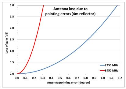
frequencies and an antenna Figure 26: Loss of antenna gain due to antenna-pointing errors
