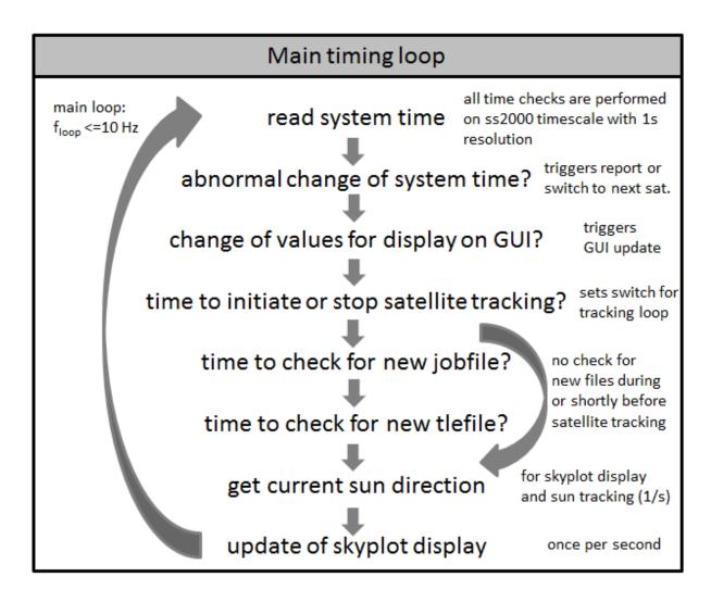
Figure 51: Layout of the main timing loop
