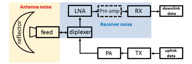
Figure 31: Categories of system noise w.r.t basic signal paths at ground station
