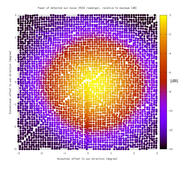
Figure 76: NYA-1 directivity w/o boresight offset compensation, square scan, 0.1° steps
