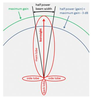
measured, calculated (modelled) or Figure 25: Half power beam width of main lobe
