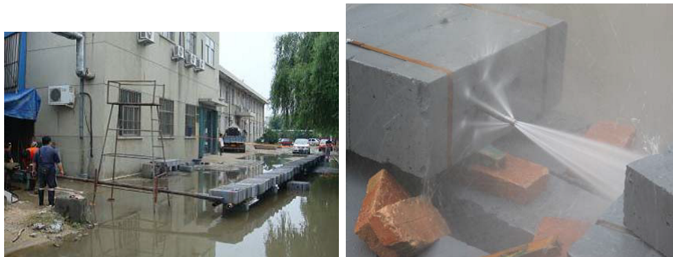
Figure 10: Yard test on porous concrete blocks (Huanpeng et al., 2013)
