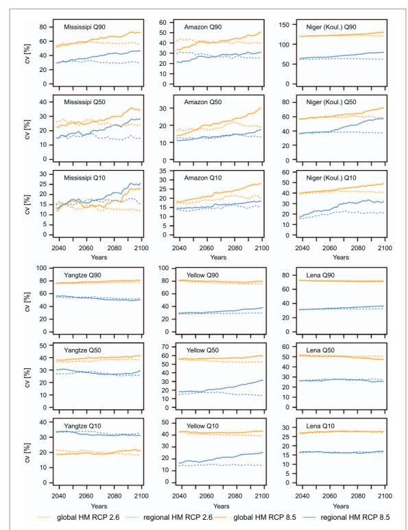
Figure A1. Variability in changes in Q50 (mean flow), Q90 (low flow) and Q10 (high flow) based on all simulation results for the RCPs 2.6 and 8.5, separately for the regional and global models (blue and orange curves) for the Mississippi, Amazon, Upper Niger, Upper Yangtze, Upper Yellow and Lena in the period 2030–2100.
