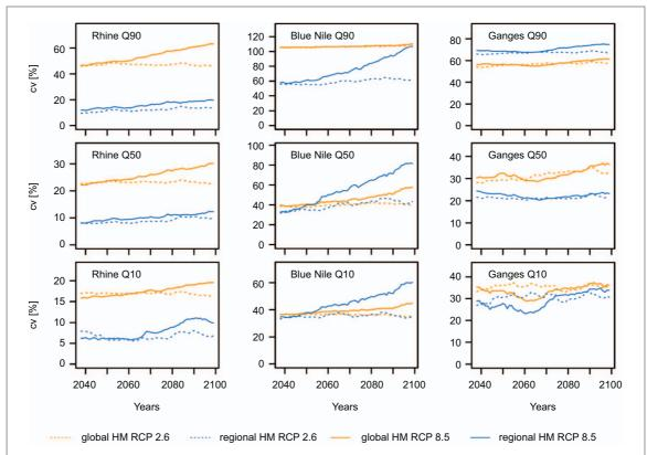
Figure 2. Variability in changes in Q50 (mean flow), Q90 (low flow) and Q10 (high flow) based on all simulation results for the scenarios RCPs 2.6 and 8.5, separately for the regional and global hydrological models (blue and orange curves) for the Lena, Blue Nile and Ganges in the period 2030–2099.
