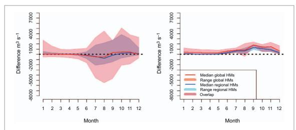
Figure 4. Range of impact uncertainty in the Niger basin (change in discharge at gauge Koulikoro comparing the long-term monthly values of the reference period 1971–2000 and the scenario period 2070–2099) using all GCMs to drive the global and regional HMs (left), and the range of impact uncertainty when the same models are only driven by one GCM (GFDL-ESM2M, right).
