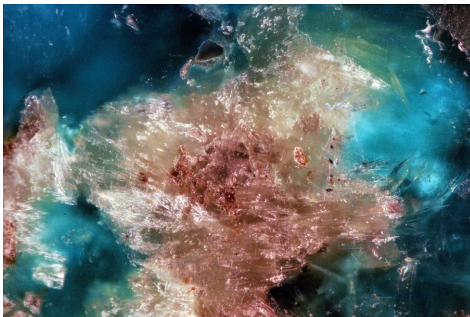
Figure 15. Detail from Se vein Type-4. Dispersed-light dark field image of an acicular aggregate of molybdomenite (colorless transparent) showing internal reflections, partly stained by inclusions of goethite (red-brown,) and surrounded by chalcocite (blue). Cacheuta is the type locality of chalcocite and molybdomenite. Width 500 \mu\text{m} .
