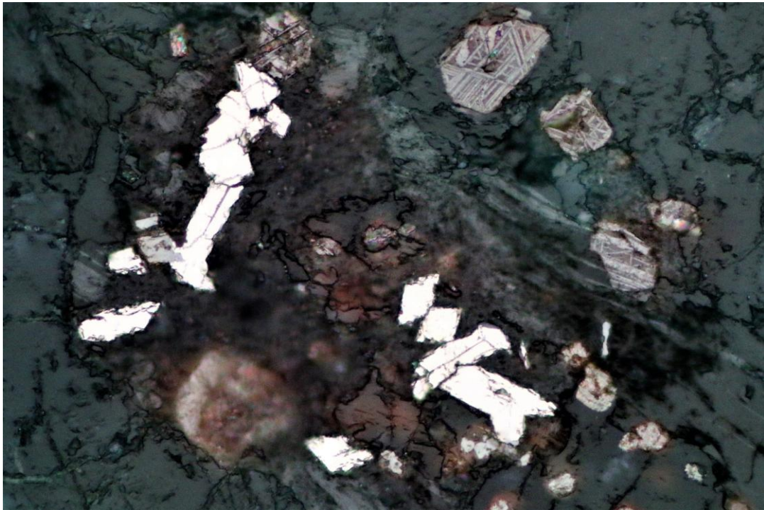
Figure 3. Single and twinned euhedral grains and radially grown crystal aggregates of ferroselite (bright cream) grown inside a host rock fragment (cf. Figure 1). Next to them (upper right) are titanomagnetite pseudomorphs (cf. Figure 2b). Polished section, plane polarized reflected light digital image, width 200 \mu\text{m} .
