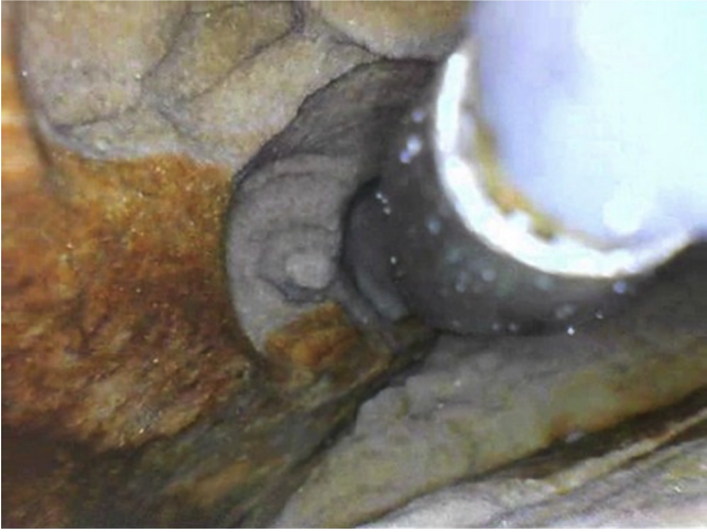
Fig. 10. Endoscopic view into the second jetted hole. The jetting nozzle hit a larger void space. Here, ROP decreased to zero and the hole was terminated.
