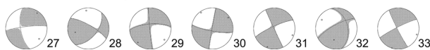
Figure 4. Full moment tensor solutions for the 33 stable events determined using the moment tensor inversion constrained to a shear-tensile source model. The lower hemisphere equal-area projection is used. Compression zones are grey-shaded and red and blue dots indicate resulting P - and T -axes, respectively.
