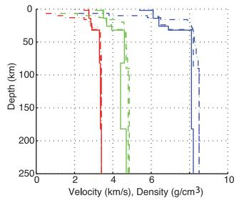
**Figure 2.** Crustal models used in the synthetic test: model S (full lines), model I (dashed lines) and model G (dash-dot lines). The figure displays  $V_P$  (blue),  $V_S$  (green) and  $\rho$  (red).
