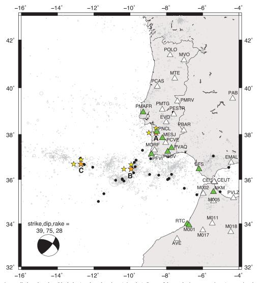
Figure 1. Map showing studied earthquakes (black dots) and used stations (triangles). Setup of the synthetic tests: stations (green triangles), test epicentres A, B and C (orange stars) and incorrect starting epicentres (yellow stars). The background seismicity in the instrumental (post-1961) catalogue is displayed by grey circles (Carrilho *et al.* 2004; Preliminary Seismic Information 2010; Pena *et al.* in press). The test focal mechanism is shown on the lower left corner.
