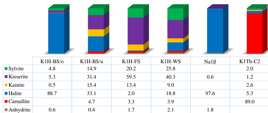
Figure 3. Mineralogical composition of test specimens (mineral concentrations in %).
