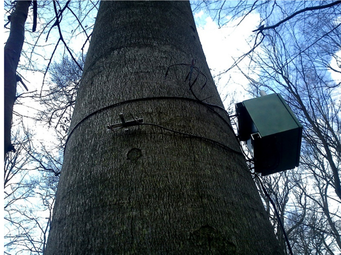
Figure 3: Old beech stem with point-dendrometer and sap-flow sensors
