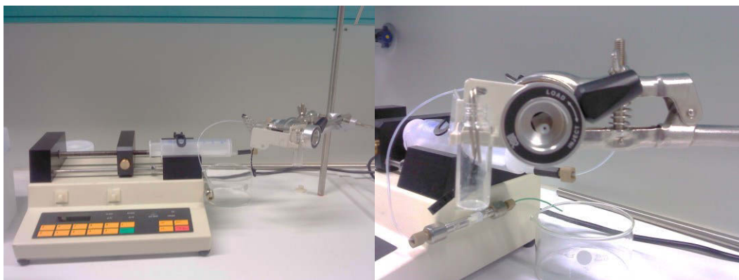
Fig. 4.20 Installation of a 200 \mu l-loop valve in the SPE apparatus. The new valve was included to reduce the variations in the amount of eluent (methanol).
