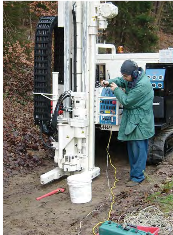
A direct-push sounding device at work
