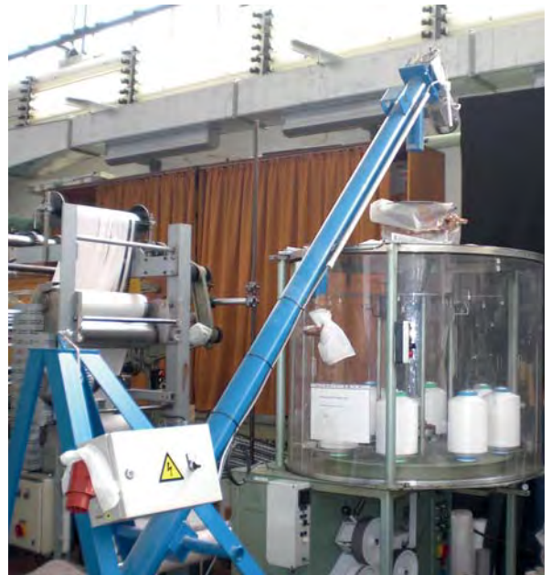
Modified R-L small circular knitting machine with feed, metering and filling equipment
