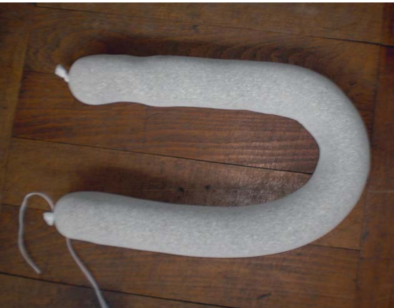
Sealant tube made from a small circular knit with integrated BEN-TONITE granulate
