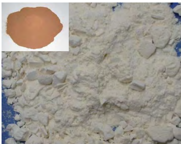
Magnesium ammonium phosphate (MAP) and sewage sludge ash (small image)
