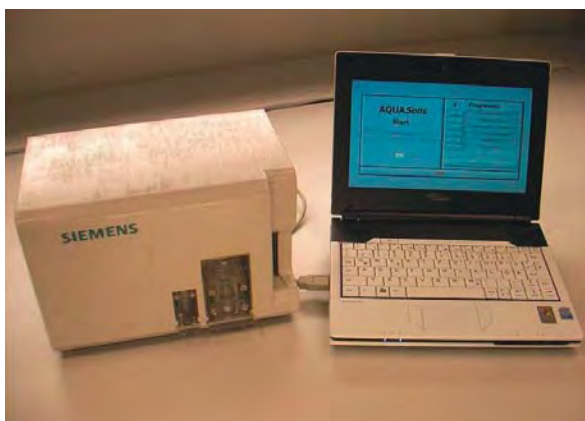
The mobile reader provides a read-out for water impurity results
