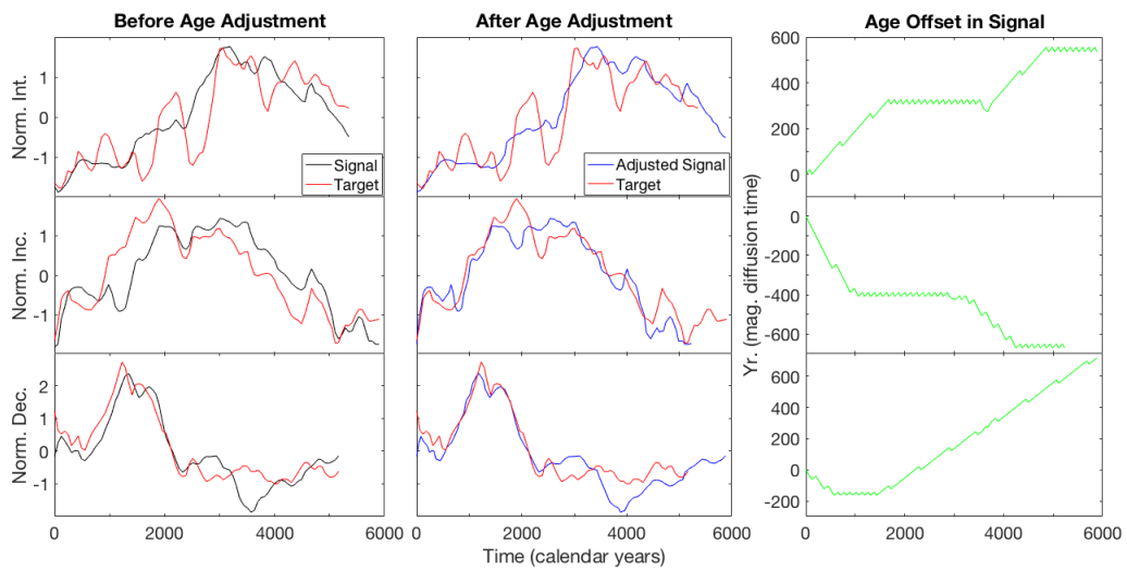
Figure 17: Illustration of correlation from numerical dynamo simulation runs for 6,000 years (based on magnetic diffusion time) during non-excursion field behavior. Signals and targets were chosen for a correlation coefficient of R \approx 0.8 . Left-hand panels are normalized field components intensity, inclination, and declination for signals and targets before running the Match-2.2 algorithm of Lisiecki and Lisiecki (2002). Centre panels are results of the match, and right-hand panels are offsets in years at each time step. Note that components have been matched individually.
