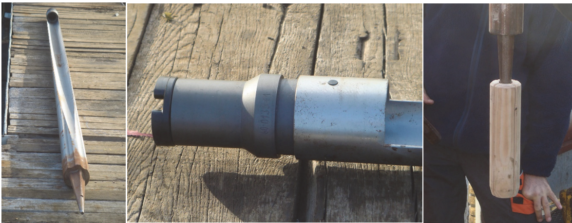
Fig.10. Components used for the sidetrack drilling: whip stock (left), technical detail of the applied mechanical setting tool (centre), wood plug as base of the whip stock (right) (Photos: GFZ).
