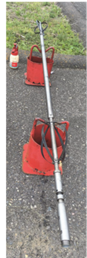
Fig. 4. MID logging tool under preparation for the last measurement campaign in May 2017 (Photo: GFZ).
