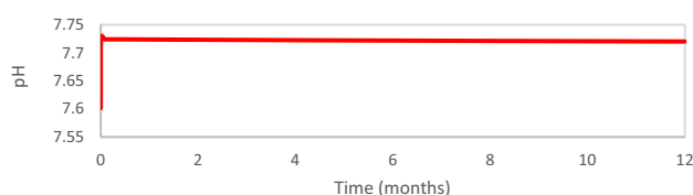
Fig. 10 The evolution of pH as a consequence of hydrogen injection within 1 year (obtained from the final kinetic model; A_{sp} specific contact area ( \text{cm}^2/\text{kg} water):1; rate constant ( \text{mol}/(\text{cm}^2\text{s}) ): 1\text{e-}7 ; injected \text{H}_2 fugacity: 7.5 bar)
