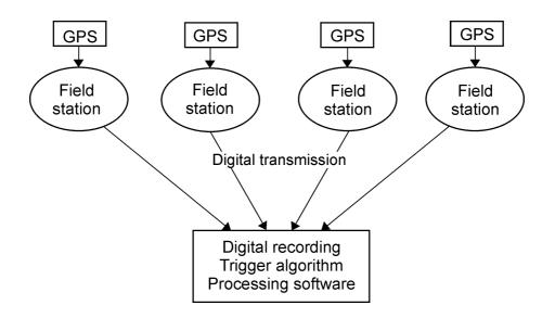
**Fig. 8.7** Typical digital network. The digital data is transmitted to the central site over fixed digital communication channels. At reception, the signals enter the recorder directly. Timing normally takes place at the field stations, although some systems also time the signal on arrival.
