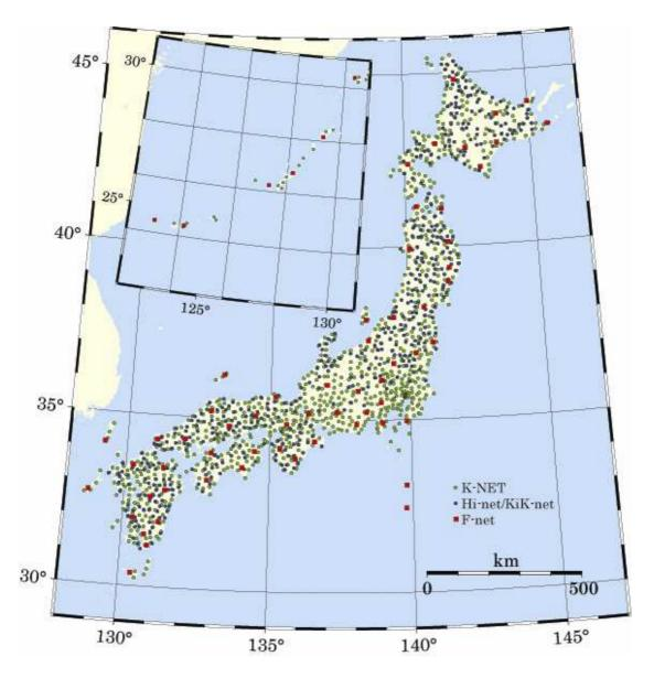
Fig. 8.14 Japanese Seismic Networks (Hi-net, F-net, and K-NET/KiK-net).
