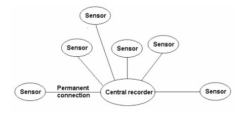
**Fig. 8.2** Scheme of a physical seismic network. The sensors are connected to a central recorder through a permanent physical connection like a wire or radio link. The transmission may be analog with digitization taking place centrally, or an analog-to-digital converter (ADC) could also be placed at each sensor and the data transmitted digitally.
