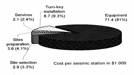
**Fig. 8.21** Cost distribution of a small, technologically high-end seismic network with an inappropriate allocation of funds.
