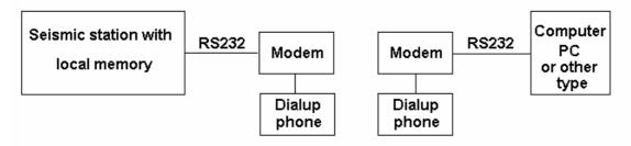
**Fig. 8.9** Manual dial-up to a seismic station for data inspection and/or download. The dialing computer can be of any type as long as a terminal emulator program, such as Hyperterminal in MS Windows, is available.
