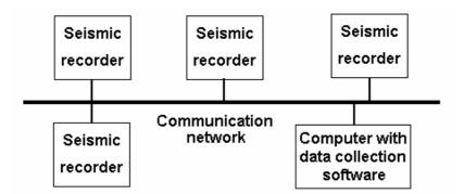
**Fig. 8.3** Scheme of a virtual seismic network. The thick line is the communication network, which can have many physical implementations. The data collection computer collects data from some or all of the recorders connected to the network.
