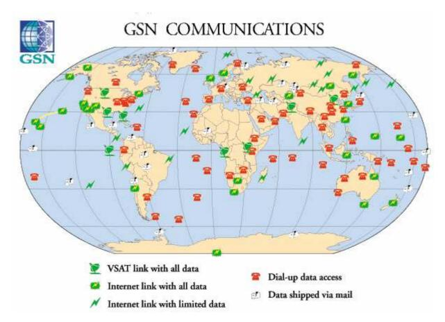
**Fig. 8.11** Communication to GSN stations 2001. VSAT is a satellite connection. VSAT and Internet have real-time connections and potentially all data can be downloaded, while the dial up stations transmit a limited amount of data only (figure from IRIS home page <u>http://www.iris.edu</u>)
