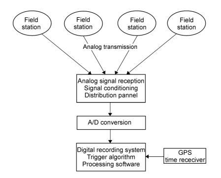
**Fig. 8.6** Typical analog-digital network. The analog data is transmitted to the central site over fixed analog communication channels, usually FM modulated radio links or phone lines. At reception, the signals are put into a distribution panel where incoming signals are demodulated. Some filtering may take place before the data are digitized by a PC or similar recording system. Timing is done within the digital system. Today, very few alternatives to GPS exist.
