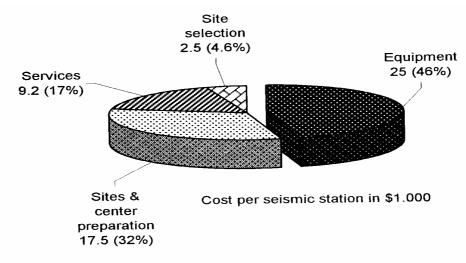
**Fig. 8.20** Cost distribution of a relatively large national seismic network with 20 SP seismic stations, strong-motion instrumentation, and analog FM telemetry.
