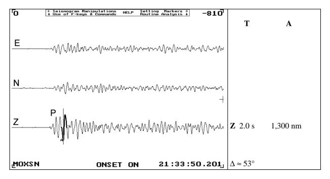
**Figure 4** As for Figure 3, however short-period (0.5 to 3 Hz) filtered record section of the P-wave group only. Note that the amplitudes are given here in nm (10<sup>-9</sup> m).
