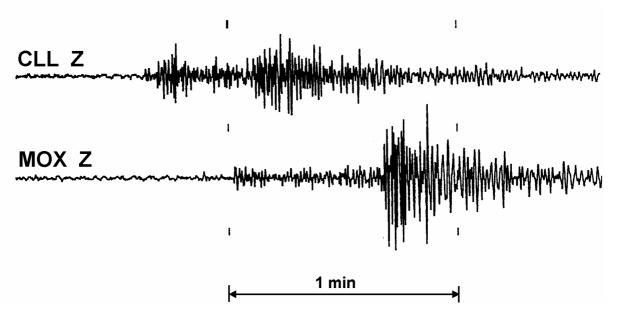
**Figure 1** Vertical component records of a local seismic event in Poland at the stations CLL and MOX in Germany at scale 1:1. The magnification values Mag(SM) as a function of period T for this short-period seismograph are given in Table 1 below.
