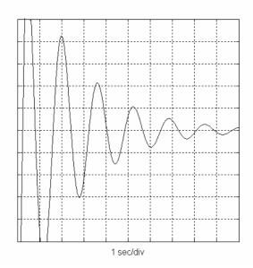
**Figure 2c** Seismometer step response: calibration coil with external resistor  $R_a = 1$  kOhm.
