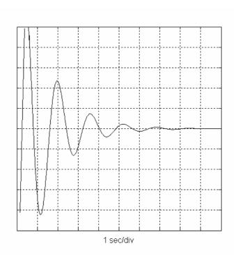
**Figure 2b** Seismometer step response: signal coil with external resistor  $R_a = 67$  kOhm.
