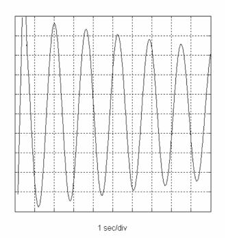
Figure 2a Seismometer step response: open circuit.
