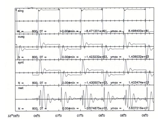
**Figure 2** The input signal is a square wave. It is used for calibration of an undamped 10 Hz geophone in a half-bridge. Note that the input signal appears in the output by coupling through the coil resistance. This would not be the case for a seismic input signal and therefore must not be interpreted as part of the transfer function.
