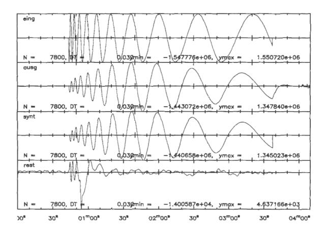
**Figure 1** The input signal into the calibration coil (eing) is a "sweep", a sine-wave whose frequency is automatically tuned from about 2 s to 50 s. It is used for calibration of a 20-sec STS1 seismometer. The second and third traces show the output (ausg) signal and the best fitting synthetics (synt), respectively. The lowermost trace is the residual signal (ausg - synt = rest).
