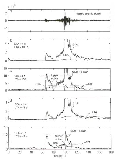
**Figure 4** Influence of LTA duration on trigger algorithm sensitivity to earthquakes containing weak P waves.
