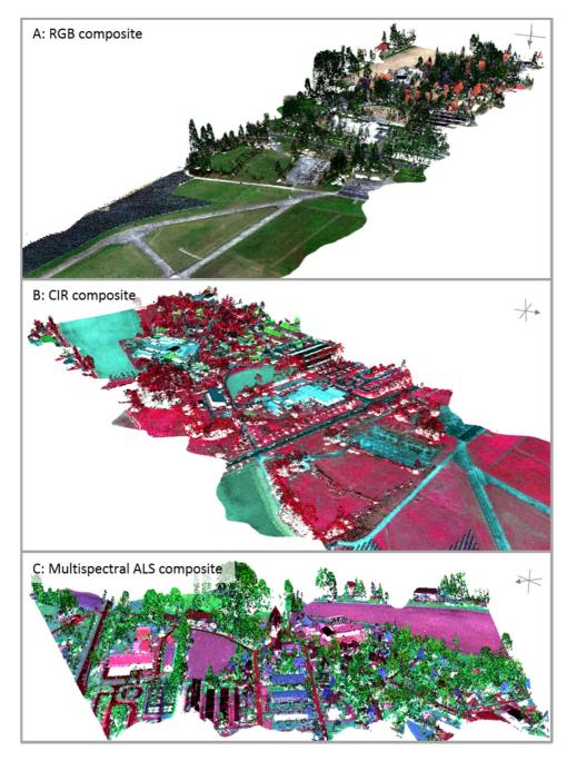
Fig. 5: Different perspective views and color composites of the hyperspectral point cloud. (A) RGB composite (R = 640 nm, G = 549 nm, B = 469 nm), (B) CIR (R = 851 nm, G = 640 nm, B = 549 nm), and (C) example of a MS ALS composite (R = 532 nm, G = 1069 nm, B = 1550 nm).
