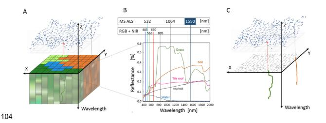
Fig. 1: Concept of the hyperspectral point cloud (HSPC). (A) ALS point cloud (first returns)
