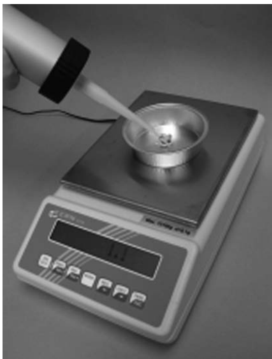
Figure 8: Measuring the cartridge extrudability of an adhesive-filler-formulation
