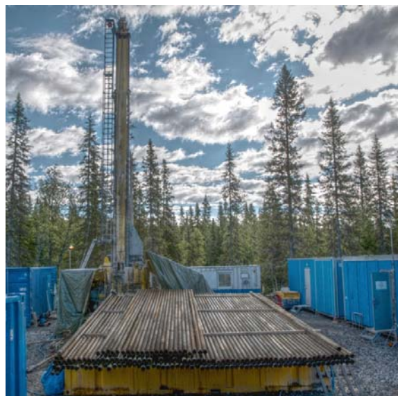
Figure 7: The “Riksrigger” drill rig with the manual pipe handling system on top of the mud tanks and c. 1400 m of HRQ drill pipe.
