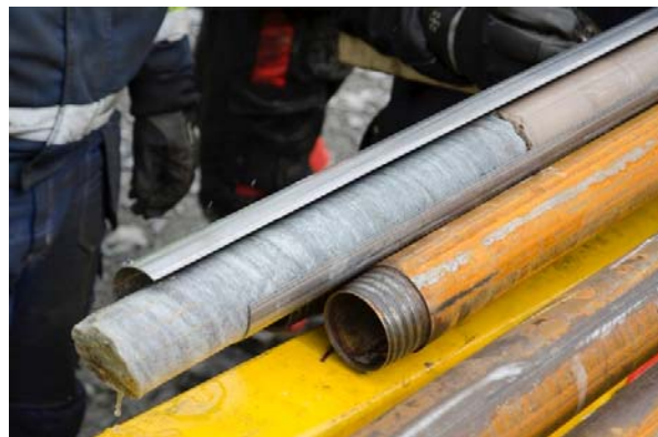
Figure 5: The first drill core (bedrock in the lower part, cement in the upper part) was pushed out of the inner tube of a triple tube core barrel assembly. Clearly visible is the split aluminium liner that protects the drill core from external forces. The second tube is also called core barrel, and the third tube is the drill string, hence "triple tube".
