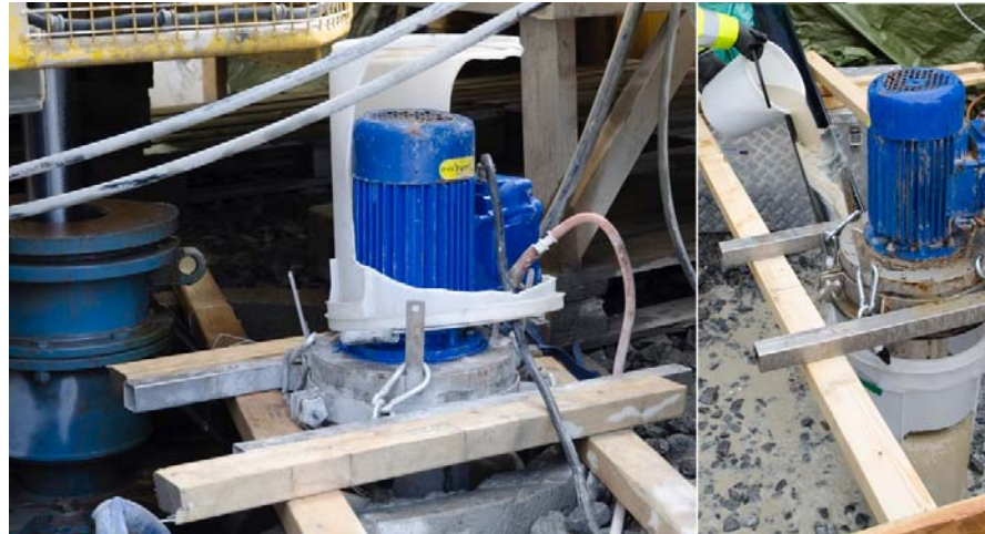
Figure 11: The OLGA degasser. The test setup to the right. A drainage pipe leads the drilling fluid into a bucket with an active volume of 10 l. The fluid is degassed by a propeller in an airtight aluminium cylinder below the electric motor and the gasses are pumped from there into the laboratory container. Under deployment to the left: the drilling fluid is caught by the drainage pipe below the wellhead and returned from the bucket via the outlet into the cellar, from where it is pumped to the settling tanks.
