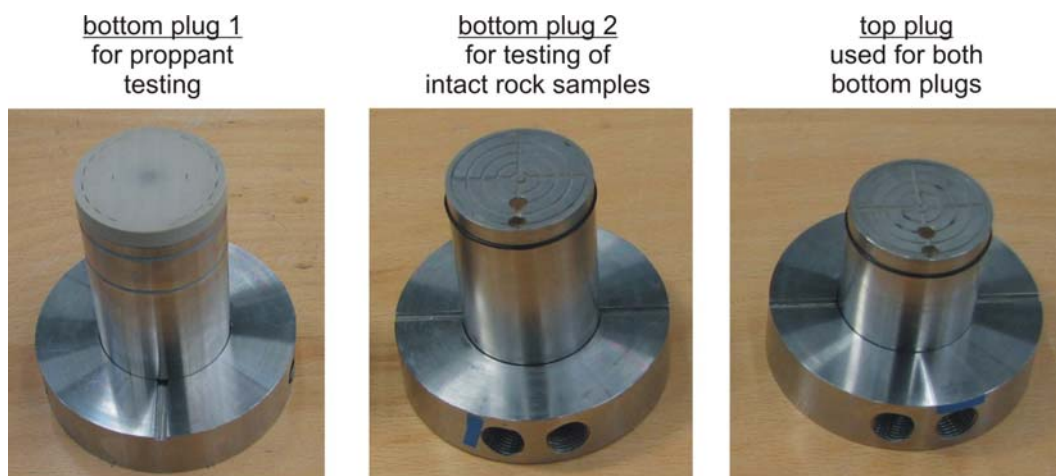
Figure 3.6: Bottom and top plugs of BDFC used for proppant testing (plug 1) and rock testing (plug 2).
